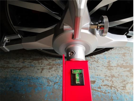
Make sure that ray positions of the rear right wheel and rear left wheel are equal. If they are not equal, move the calibration board to the left or right horizontally, as shown in the figure:
